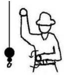
**CRAWLER CRANE TRAVEL, ONE TRACK** – Indicate track to be locked by raising fist on that side.
