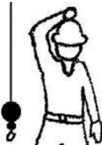
**USE MAIN HOIST** – A hand taps on top of the head. Then regular signal is given to indicate desired action.
