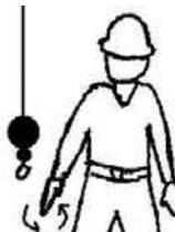
**LOWER** – With arm and index finger pointing down, hand and finger make small circles.
