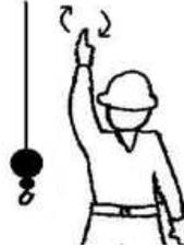
**HOIST** – With upper arm extended to the side, forearm and index finger pointing straight up, hand and finger make small circles.
